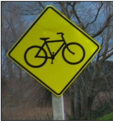
Figure 93: PW-35 (MOTSAM) / W16-7 (TCD Rule) permanent warning sign for motorists
